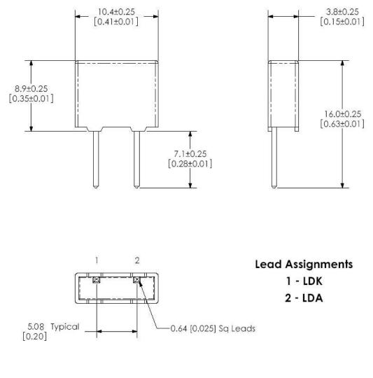
Notes: 1. Dimensions include Mold Flash 2. Controlling Dimensions are in Inches 3. Dimensions are shown in mm [inch]
